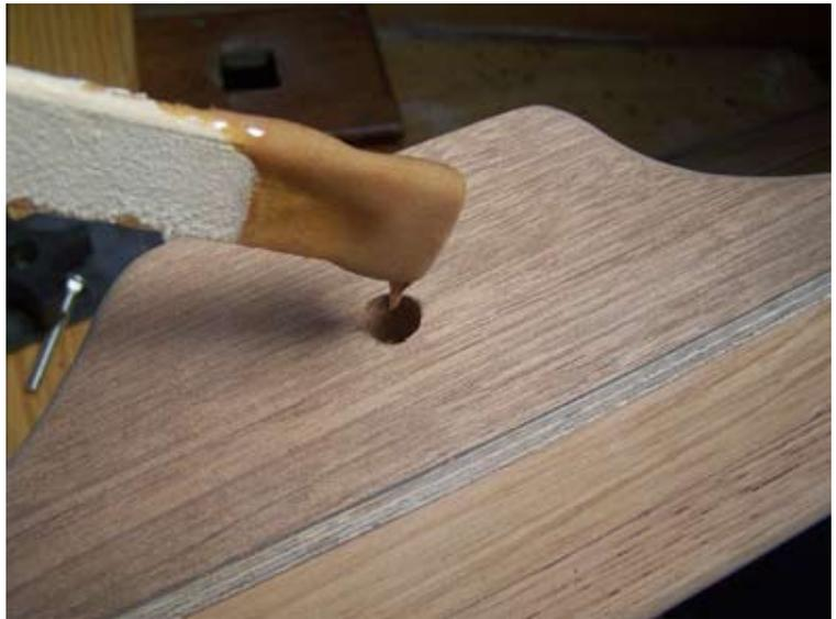
When the epoxy-filled holes have cured, sand them smooth.
