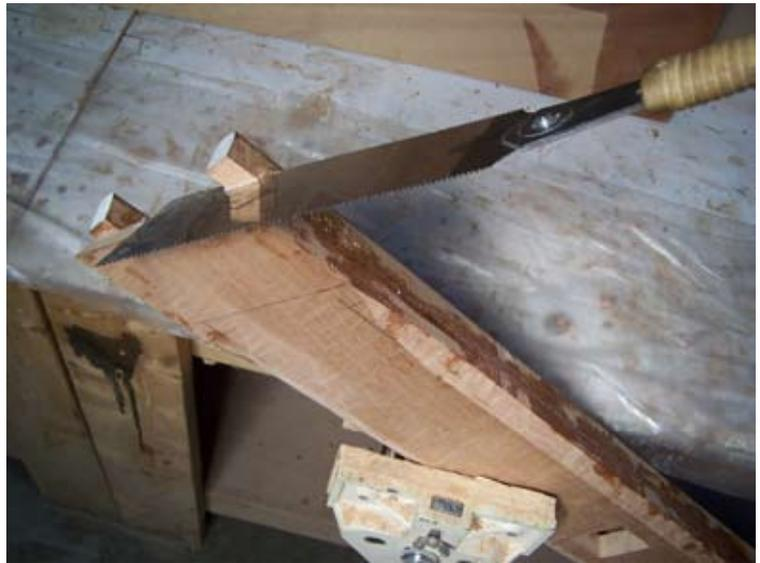
We rounded the ends of the stringers, using an epoxy filler can as a pattern.
