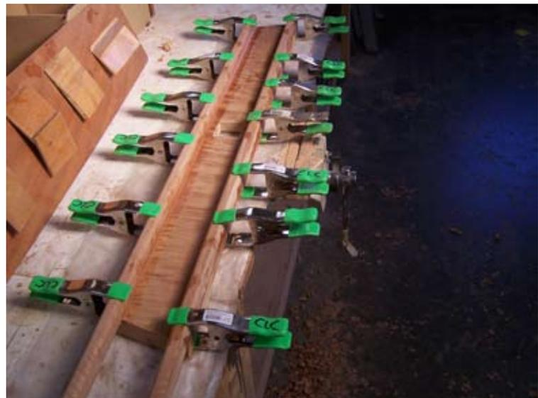
Double-check and triple-check against the boat that your thwart is the right length and that the angles are correct, then trim the thwart assembly to length.
