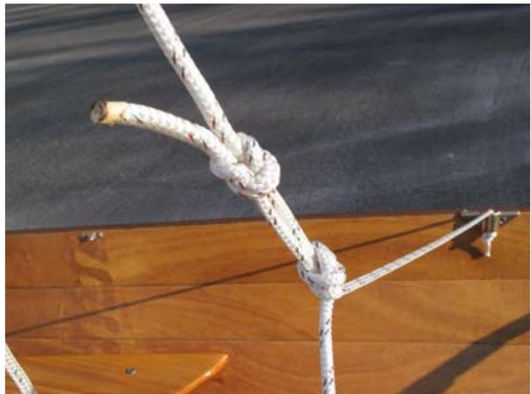
The mainsheet is rove through two single blocks lashed to the boom. Use 1/8" (3mm) line to lash the blocks to the boom.
