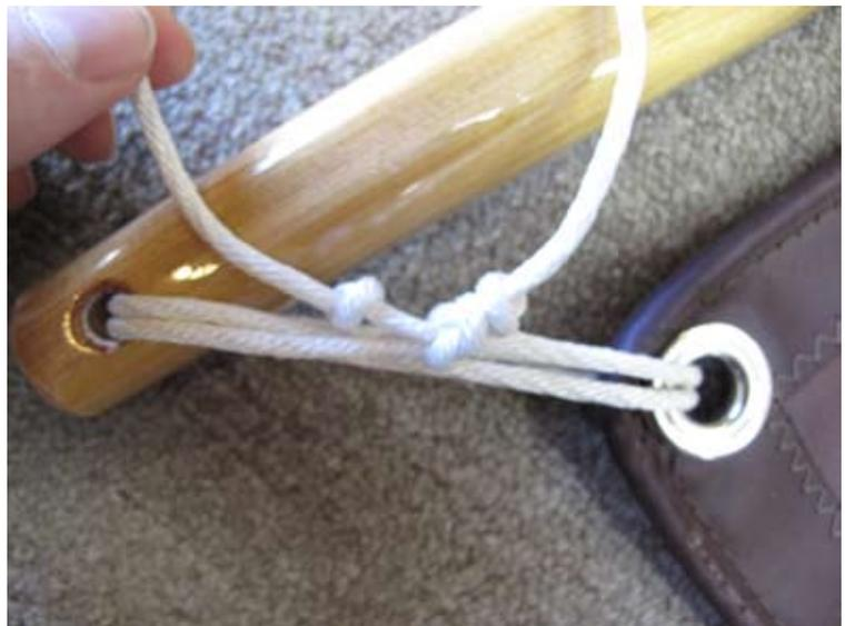
Each grommet on the head and foot of the sail is lashed around the spar. We used two loops each. These lashings should be tight enough to bring the sail in solid contact with the spar, but not so tight that the tension of the sail can’t be adjusted with the outhauls.
