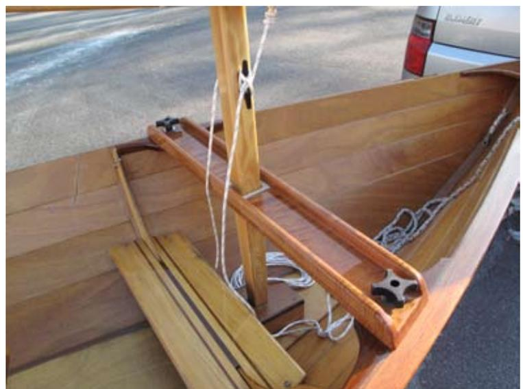
A view of the halyard in action. You should hoist the sail first with the halyard, then take up on the downhaul.
