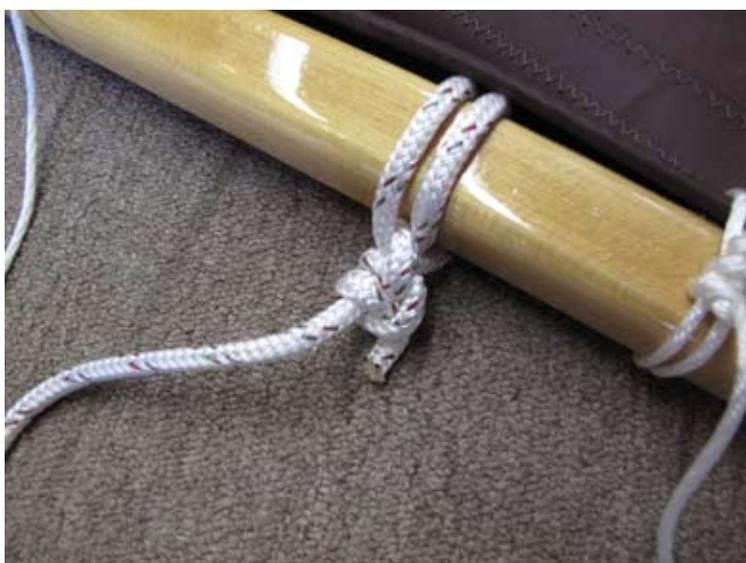
Use a hot-knife to cut off all of the excess lashing line, right up against the stopper knots.
