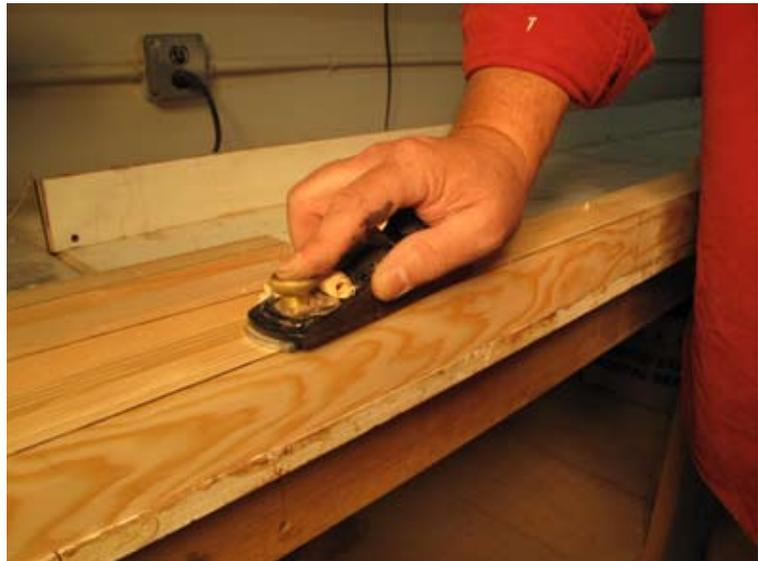
The square-sectioned mast is ugly and heavy with sharp corners. We used a router with a 1/2-inch round-over bit to knock the corners off. This looks great, and saves a lot of weight where it matters the most---up in the air.
