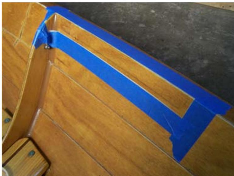
Every trace of varnish must be sanded away if you're retrofitting. If you're working on a hull that just has an epoxy coating, you still must scuff up the mating surfaces for the strongest-possible bond.
