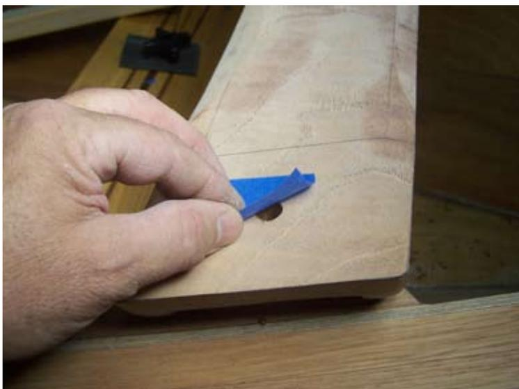
The thwart knees get the same treatment: a bit of tape on the underside, then a solid fill of thickened epoxy.
