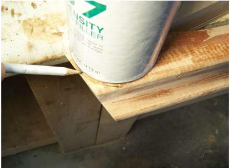
For extra strength, we recommend that a “peanut butter consistency” epoxy fillet be added to the underside of the thwart knees.
