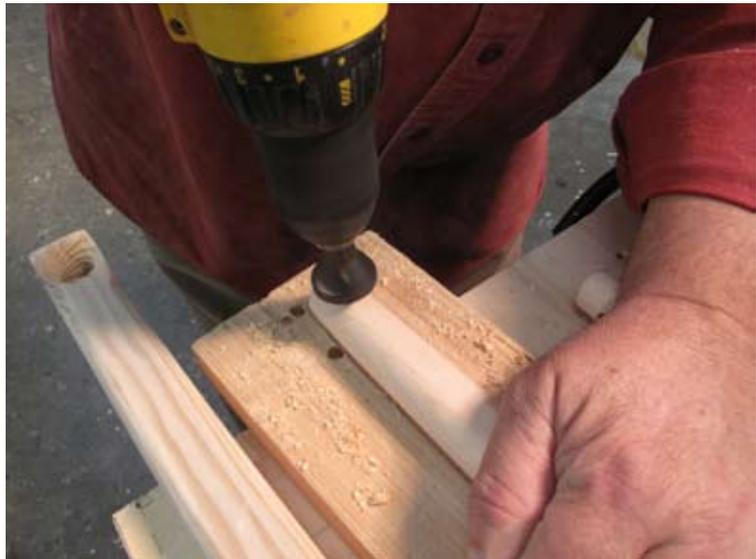
The finished hole, with a neat “flare” to prevent friction on lashings.
