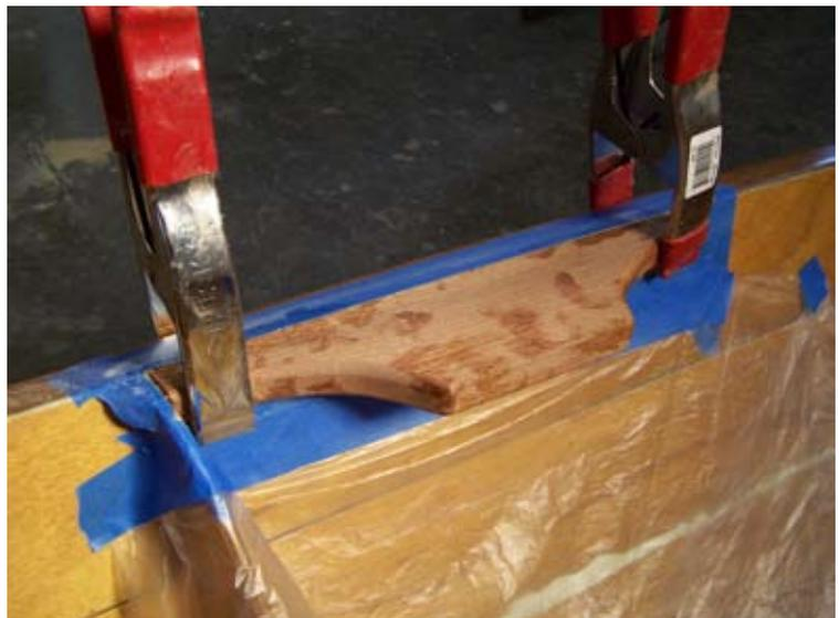
Note the trouble we took with plastic and tape, to avoid dripping epoxy on the varnished interior of our showroom model.
