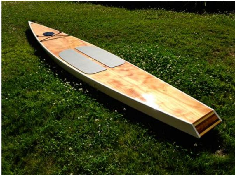
The Kaholos are okoume marine plywood, stitch-and-glued together, sheathed in fiberglass and epoxy, with a grid of bulkheads and stiffeners inside to make the boards stiff and light. With a week to spare you can have a completed board and be out on the water before you know it.
