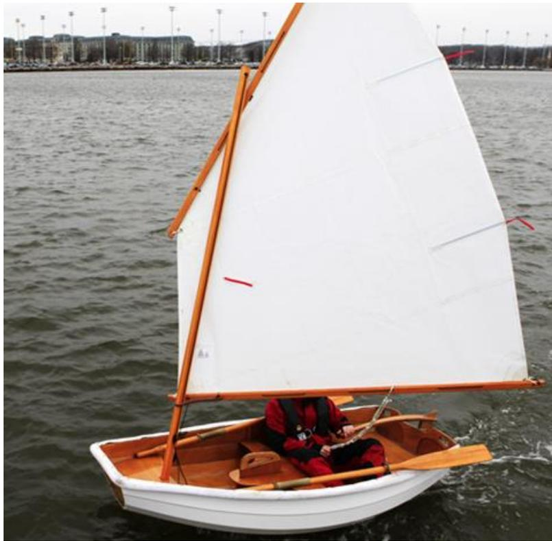
The Eastport Pram's many joys are multiplied when you add the sailing rig. Not a clumsy add-on, the large standing-lug sail and efficient rudder and daggerboard convert the pram into a proper sailboat with enough real performance, upwind and down, to keep the most seasoned sailors interested. The 48-inch beam means that the likelihood of capsize is remote as long as the sheet is never tied down. This is the perfect craft in which to learn to sail, whether the crew is age 8 or 80.
