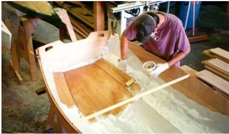
For all its virtues, perhaps the neatest thing about the Eastport Pram is the ease of construction using CLC's patented LapStitch process. Not only does the hull go together in a single weekend, but everyone agrees that the lapstrake Eastport Pram is one of the most beautiful dinghies they've ever seen. It will take the patient novice only 40-50 hours to assemble the hull, with a little more part time work for finishing. It is one of CLC's easiest kits and perfect for families.
