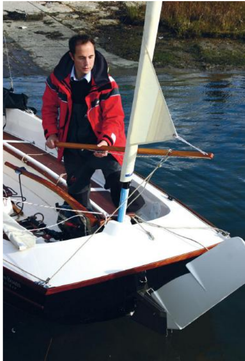
Rigging the mizzen, which is sleeved around a windsurfer's mast. The step in the rudder allows boarding from the water; the assembly is engineered to take the weight
