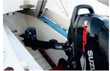
Flexible plastic fairing strips help to reduce turbulence in the outboard well
