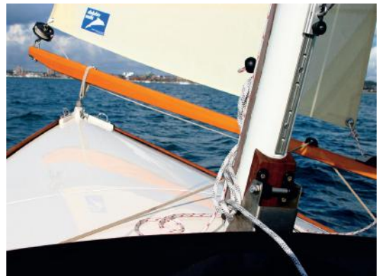
The mast (painted carbon/glass in this case) is stepped in a tabernacle. A self-tacking jib is optional
